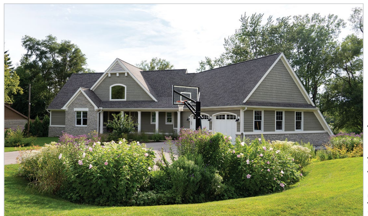
Rain gardens can be placed anywhere but are most efficient near driveways and other hard surfaces that don't allow rainwater to filter through them.
